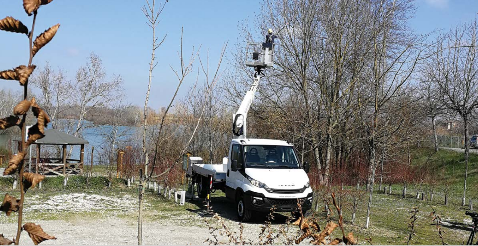
Scorpion 1490 has a telescopic boom that's operated by simple, intuitive proportional controls
